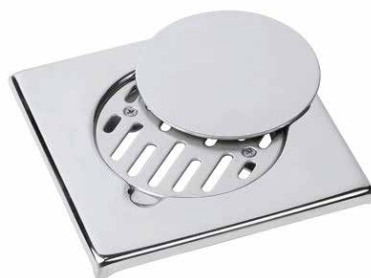
Floor drain with screwed grate and cover plate Vertical outlet ø 103mm AISI 304 20*20
